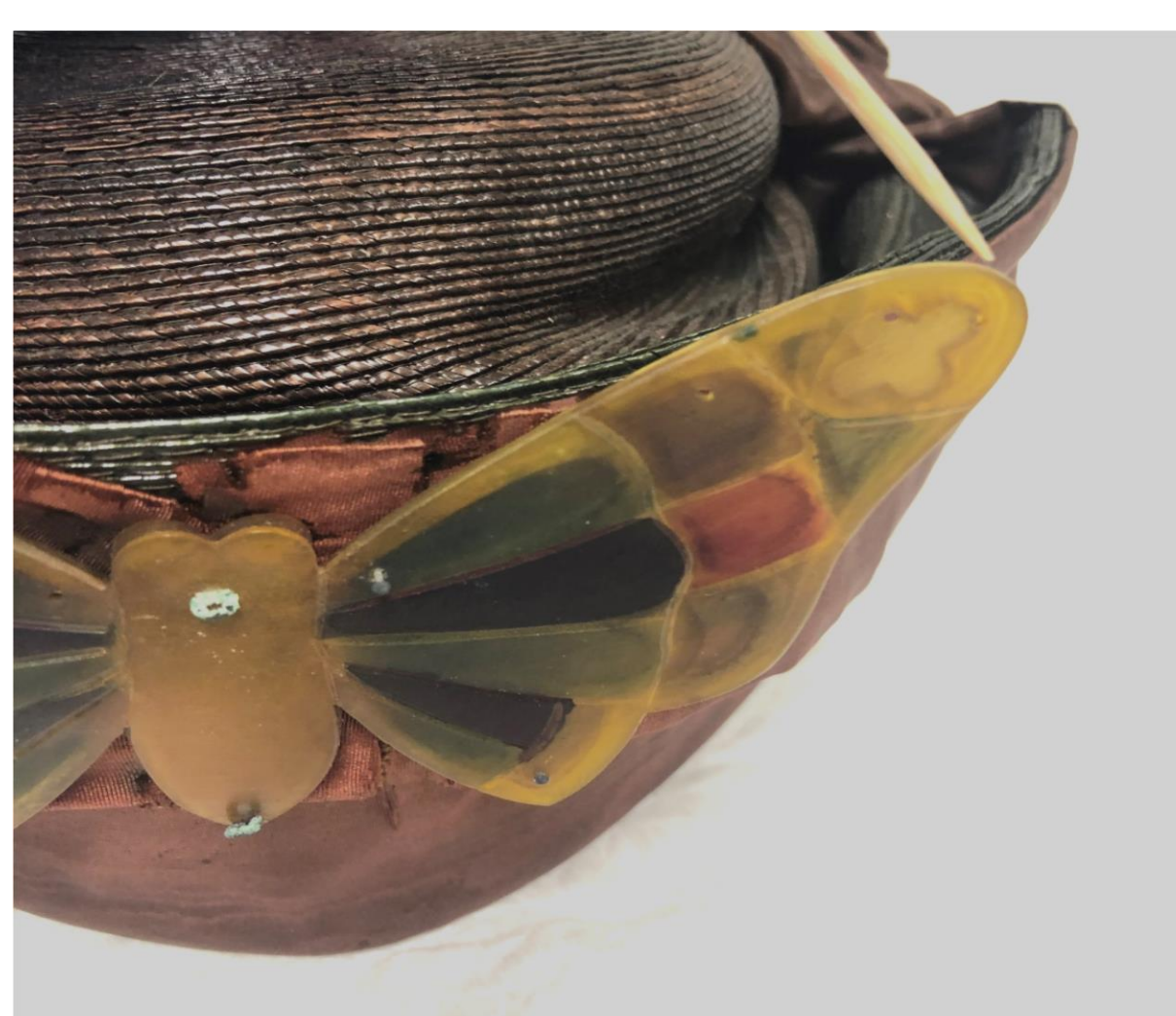
Cellulose nitrate hat ornament. Pointer shows area of FTIR analysis.
